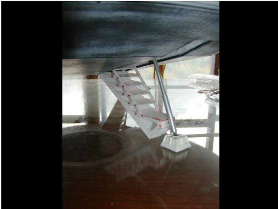
When you're happy with the operation of the gear, install the top of the gear well. It is best to paint the interior of the wells before attaching the top.
