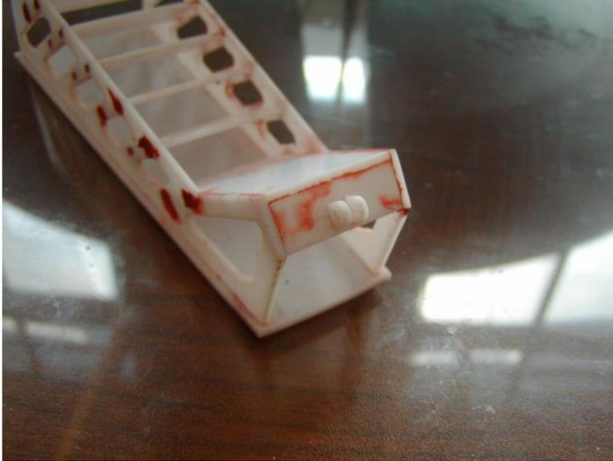
Ensure a good glue joint on these parts as this will be the connecting point between the landing gear and the gear strut.
