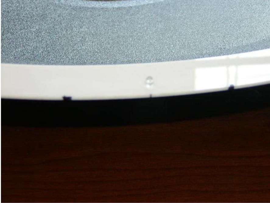
Attach the upper hull half to the upper ring. Align the center the hull with the mark made on the ring half. Make sure to center the hull half on the ring. Align the mark with the center of the main view port. See picture.
