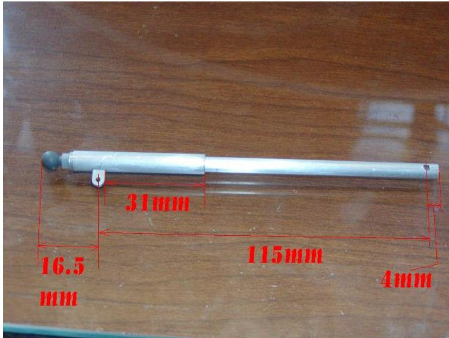
Measure up 115 mm and drill a small hole through the top of the strut. This hole should be at a right angle to the 'D' ring. This will be for the T bar, made from a piece of wire coat hanger.
